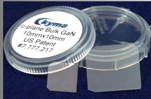
Free standing GaN 10mmx10mm and 18mmx18mm substrates
