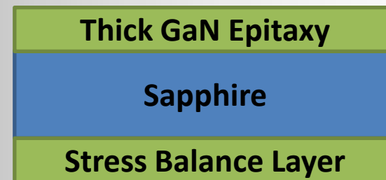
Typical FLAAT template structure
