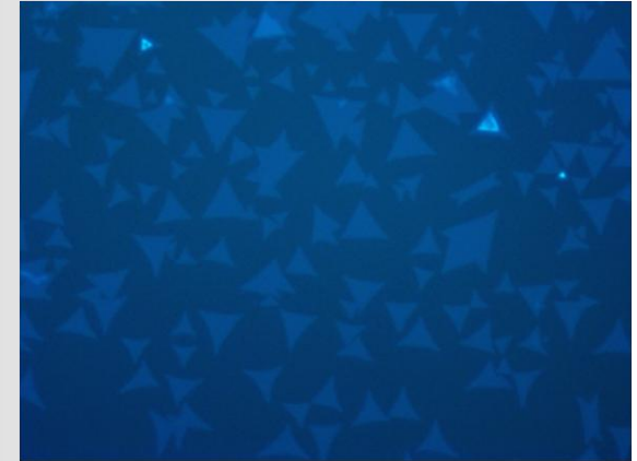
Monolayer MoS2 crystalline grains produced at Kyma
