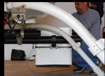
Radiometer prototype installed for aerial deployment
