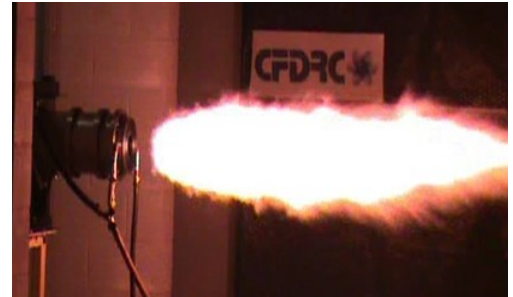
Successful hot-firing of ATR system
