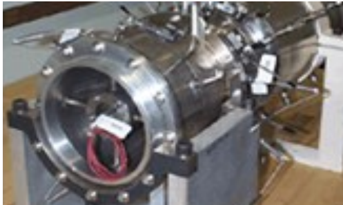
Air Turbo Rocket assembly
