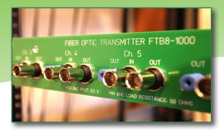
**EHT Fiber Optic Isolators** provide fiber optic high voltage isolation to TTL-type control signals for robust noise immunity. Multichannel fiber recievers include relays for actuating interlocks.
