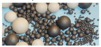
IST has incorporated the hollow shells into both metal and polymer matrices for armor, structural and buoyancy applications.
