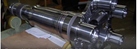
The power of the forward rotor shaft of Boeing's CH-47 Chinook helicopter is expected to be increased by 15% or more by replacing incumbent 9310 steel with stronger, tougher Ferrium C61. A C61 forward rotor shaft is shown at right undergoing rough machining.
