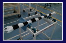
Ferrium M54 offers ultra high strength and tough ness for use in demanding applications such as the hook shank for the Navy's T-45 aircraft. In 2013, the Navy qualified M54 hook shanks (one pictured above) with more than twice the service life over incumbent Hy-Tuf steel. QuesTek is serving as the prime contractor and will deliver 40 components in 2016, with a cost savings to the Navy exceeding \$3 Million
