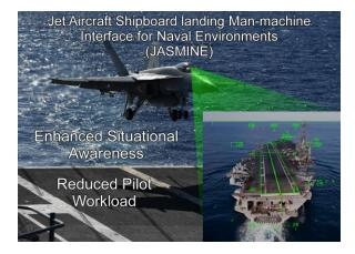
New guidance algorithms and display symbology leads the pilot to the desired approach and recovery. For Navy strike fighter pilots, JASMINE will reduce pilot workload and enhance safety when outside visual cues are not available under these challenging conditions. JASMINE will meet Navy objectives via a software solution that is compatible with the existing cockpit head-up display of the F/A-18E/F thereby allowing for rapid fleet integration.
