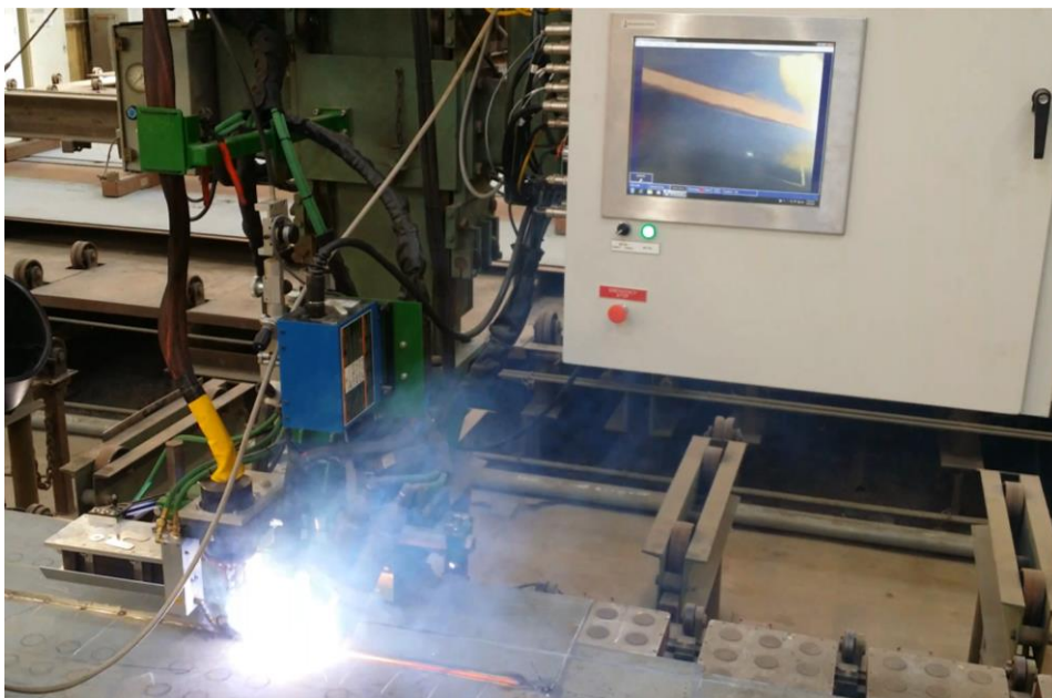
HiDep™ welding system joining 4.5mm EH-36 Marine Steel (Equivalent to ASTM A709 Grade 50). System is installed at Bollinger Shipyards, LLC, which produces the U.S. Coast Guard Fast Response Cutter ship.
