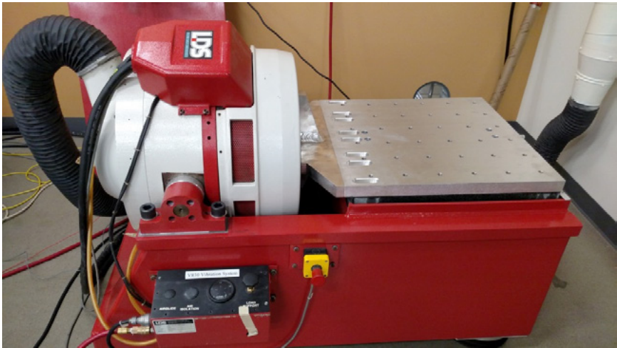
▼ ATA's in-house shaker capable of testing small and medium sized components
