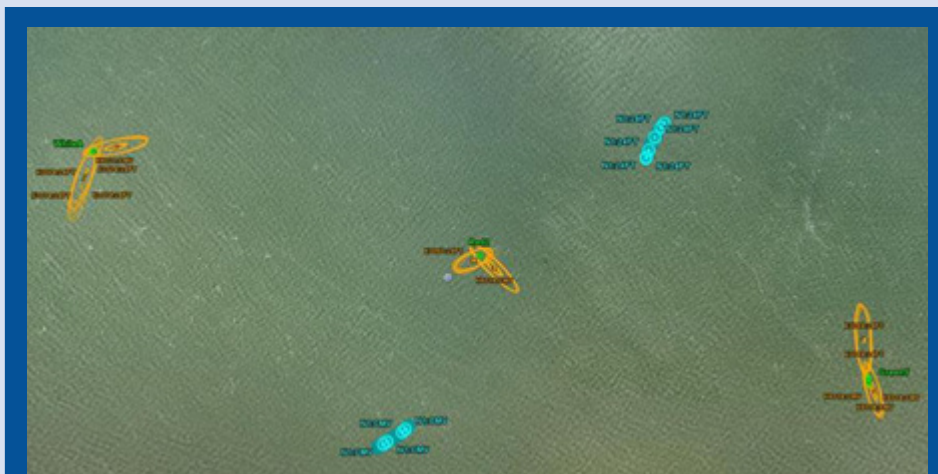
Common Operational Picture Generated in Real-Time at Sea Using Data from Two Heterogeneous USVs (fused ellipses are green (based in fusing Ka-band radar from both USVs with DNC buoy data), raw Ka-band radar is orange, USVs (CMV and 7mt RHIB) are blue) Note: Time Slice (~10 seconds) on historical Google Earth image Note: Scale ~0.4 NM x 0.75 NM
