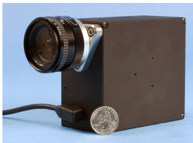
VNIR-90 - 90 Waveband Visible Spectrometer Captures hyperspectral datacubes at a resolution of 55x44 spatial by 90 spectral at video rates.
