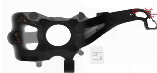
Finding patterns by mapping defects over large sample sizes of parts
