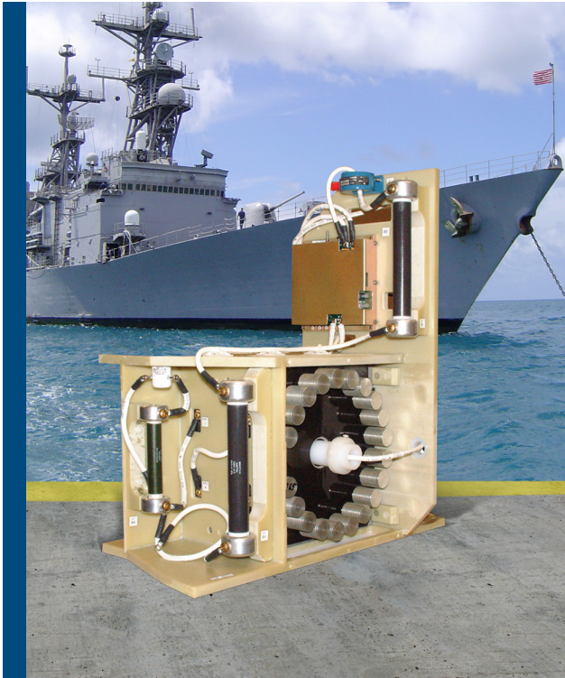
This solid-state cathode modulator assembly replaced the entire mod-anode modulator and crowbar circuit for the AN/SPQ-9A.
