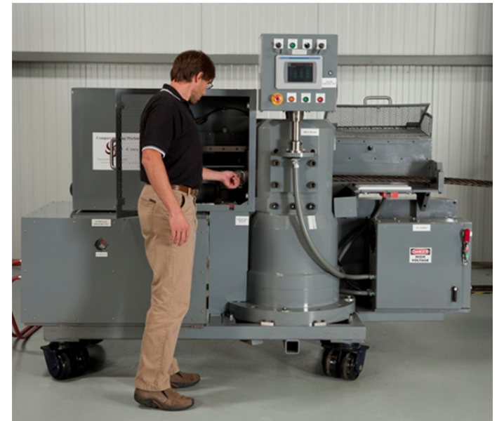
Compact Swaging Machine for Aircraft Carrier Purchase Cables
