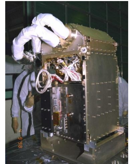
Creare-Built NICMOS Cryocooler before Installation on the Hubble Space Telescope
