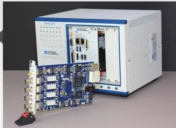
Prime Photonics FOCIST™ Data Capture Card (DCC – foreground) with Data Capture Unit (DCU - rear)
