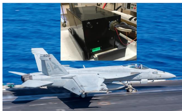
EIC 28V/25Ah Li-Ion Battery for Navy F/A-18
