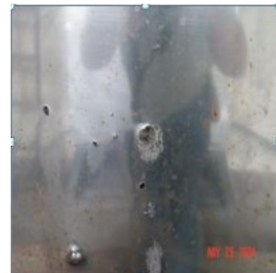
Plate perforated but not damaged
