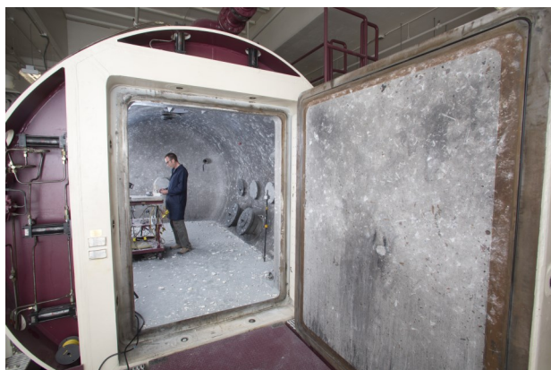
Our tests in SNL blast chamber that can handle up to 1 kg TNT
