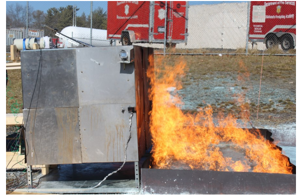
BlazeTech simulated cab subjected to a large-scale pool fire
