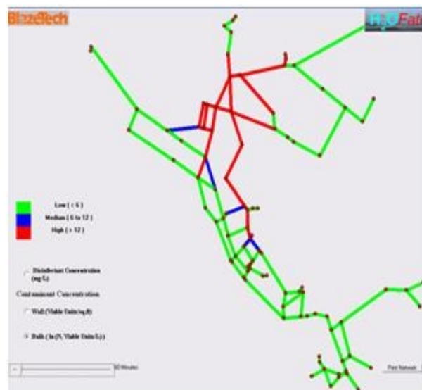
Hazard contours (red) after contaminant release into a drinking water distribution network .
