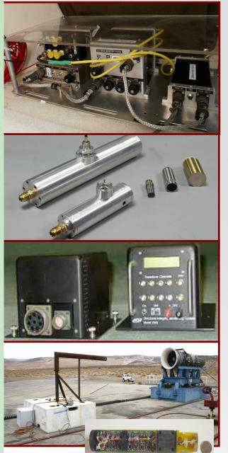
In-situ aircraft **Wiring Sensor System** for monitoring precursor damage such as wire chafing. Size, weight and power are key attributes for aircraft deployment.
