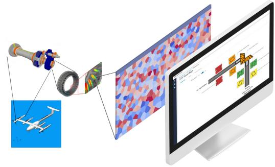
Using DigitalClone, complex system-level drivetrain models, can compare up to six sub-component variations with up to 3 different sub-component upgrade options to evaluate the optimal bill of materials configuration to improve the sustainability of the system. The computational models can be parameterized for large-scale batch simulation and data extraction using Sentient's extensive materials and component library.
