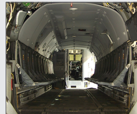
An executive-level VIP cabin liner kit was developed and produced by Kennon for the HMX-1 fleet of V-22 support aircraft (SBIR project)
