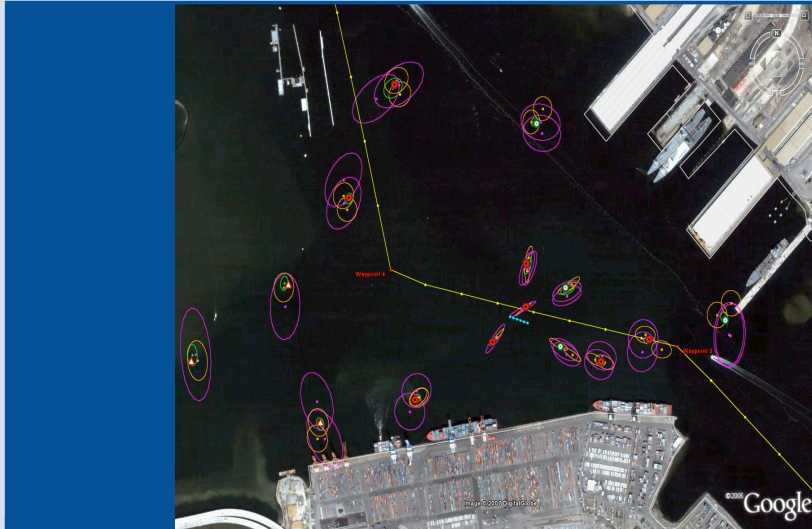
Object Avoidance Situational Awareness Screenshot (Sample Google Earth display of "World Map" data). Note: small red and green circles are Digital Nautical Chart (DNC) buoys/markers; green ellipses are from the Fused Tactical Picture (FTP) generated by Wagner's Data Fusion Engine (DFEN), other colored ellipses are raw sensor reports on buoys/markers; cyan dots show current Unmanned Surface Vehicle (USV) position along yellow waypoint track.
