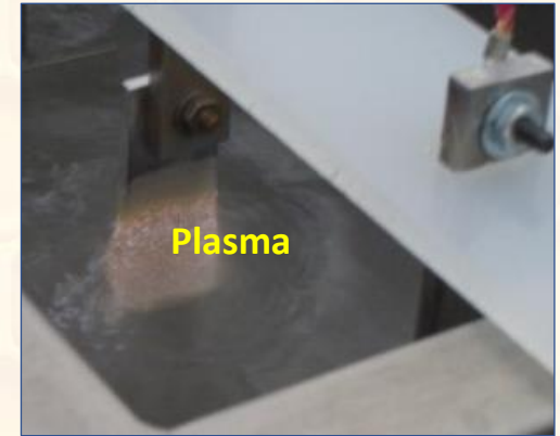
PED processing of Al test coupon
