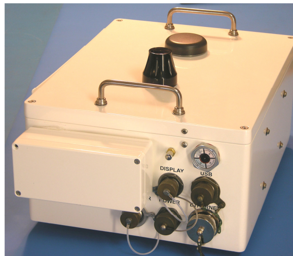
Prototype Hermetic Profiler 18 x 30 x 45cm, 17 kg, 30 watts
