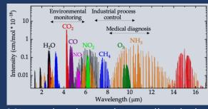
QCL wavelengths match up well with the "fingerprint" regions of the infrared where most molecules have unique, fundamental absorption features [1]. High power QCLs enable detection from a distance.
