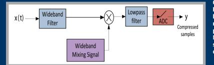
Compressive sensing overcomes the ADC bottleneck by allowing the processing of wider bandwidths with current ADC limitations. GIRD's novel random mixing approach provides a properly randomized signal with only sub-Nyquist rate devices such that the compressed samples can be processed using GRID's custom dictionaries.
