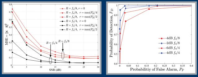
MSE of waveform reconstruction error vs. SNR for compressive sensing at two different sub-Nyquist sampling rates with different algorithm parameters. Right: Receiver operating characteristic (ROC) curves for pulse detection with different sub-Nyquist sampling rates at low SNRs.
