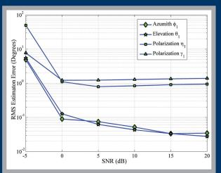
RMS errors for DOA and polarization estimation versus SNR. DOA performance at low SNRs improves significantly with longer processing frames, with DOA errors as low as 0.1 deg at -5 dB SNR.
