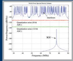
Spectra of signal of interest and SOI in a high-dynamic range scenario. SOI is below the quantization noise level for digital interference cancellation. Right: Digital cancellation of a strong interferer without a reference signal (i.e., blind) for an ideal(red) and 8-bit quantized (green) scenario.
