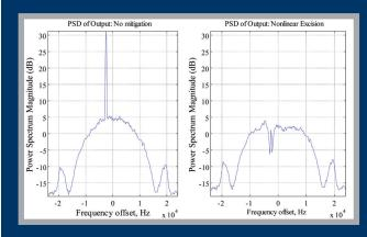
Power spectrum of signal of interest with narrowband, in-band interference (left) and cancelled interference (right). Multiple interferers can be removed simultaneously.
