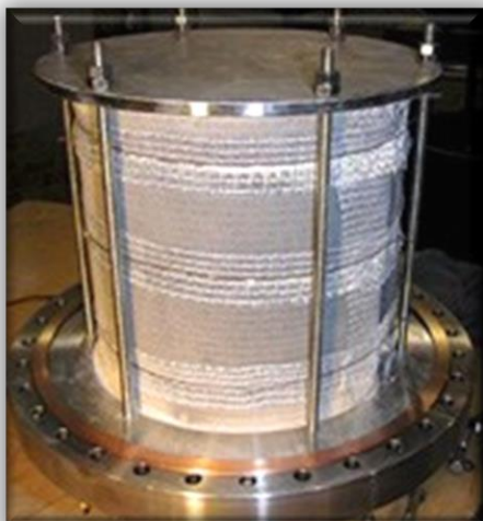
Trace Contaminant Absorber
