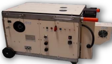
1 kW Fuel Reformer/Fuel Cell System
