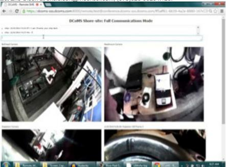
A video freeze-frame view from the SME's computer screen in his office while the SME and remotely located technician were discussing a pump's vibration level just prior to shutdown. The upper right photo is the view from the technician's head-mounted camera as he looks at the machinery space laptop (MSL). The lower right view is the upper part of the still frame bearing inspection image that had already been sent to the SME.
