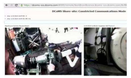
Left - A video freeze-frame view from the shore-site SME's computer screen as the SME ensures that the accelerometers for the vibration measurements are in the correct location prior to pump start-up. Right - dial indicator inspection photo previously sent to the SME during the alignment process.
