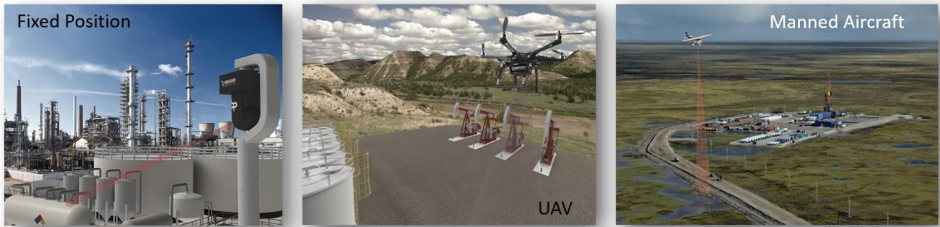
Figure 1. Gas Mapping LiDAR applications and concept of operations. (Left/Center) Short range applications such as automated facility monitoring from fixed position or UAV-mounted sensors. (Right) Long range applications such as pipeline and associated infrastructure monitoring from a manned aerial vehicle.
