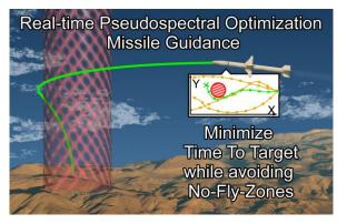
The pseudospectral optimization technology provides optimized path updates to the missile in flight, allowing course corrections to avoid and react to existing and emerging threats.
