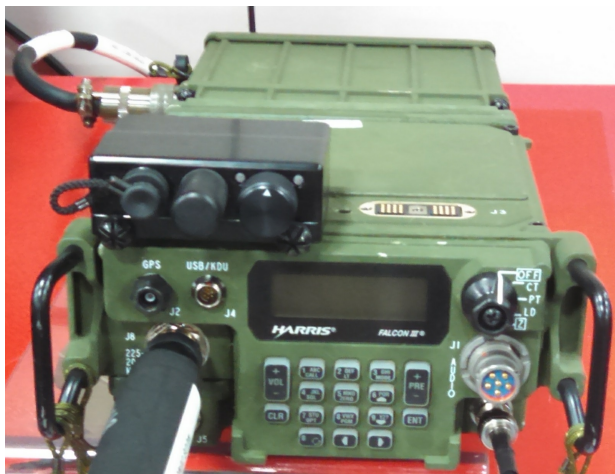
DataSoft RAP attached to Harris PRC-117G radio.
