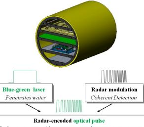
Radar transmission/detection in an underwater environment
