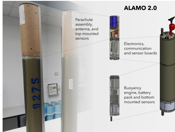
Photo of current ALAMO floats with parachute & sensors inside cardboard at top, plus inset of ALAMO-2 design model. (Copyright 2020, MRV Systems, LLC)
