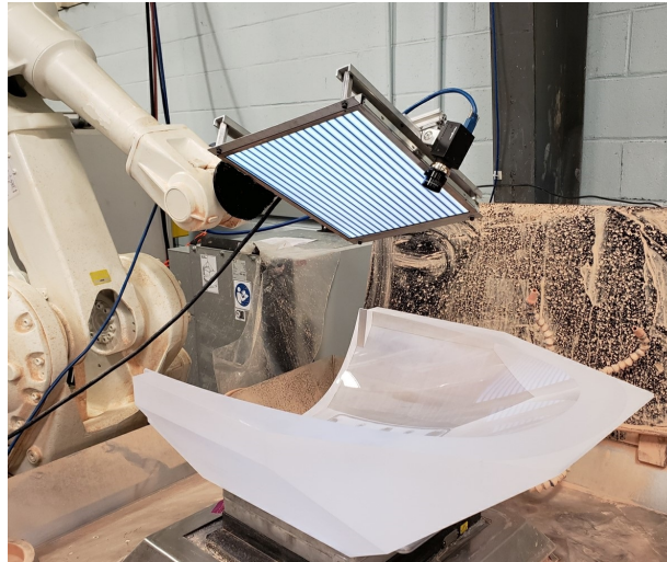
Robotic platform taking mid-spatial frequency error measurements using deflectometry in-situ on a 580 mm freeform optic (Copyright, 2018, Optimax)
