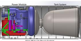
Above CAD view image depicts API's oxygen source (shown blue) as it fits into the Integrated Power System. Other main elements include hydrogen generator (purple), SOFC Fuel Cell (red), and fuel/reactant tanks (grey).
