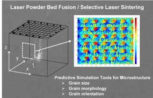
Copyright 2017 3DSIM, LLC Predictive Simulation Tools for Additive Manufactured Parts: Prediction of Part Microstructure
