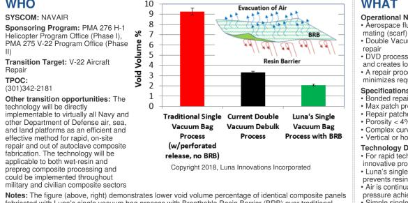
fabricated with Luna's single vacuum bag process with Breathable Resin Barrier (BRB) over traditional single vacuum bag and baseline Double Vacuum Debulk processes
