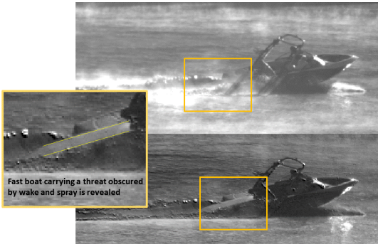
Hydra's Multi Spectral Sensor Fusion at range to enable situation awareness for Fast Inshore Attack Craft
