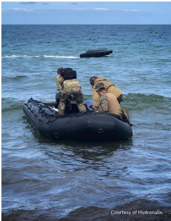
NIX, an autopilot-controlled USV, can haul gear and run resupply missions.
